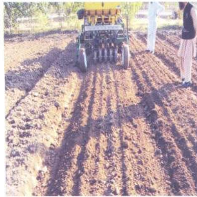
Figure 7:Wheat sowing using PRB machinery
